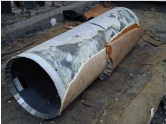
All locks remained engaged and there was no evidence of damage to the steel core.
